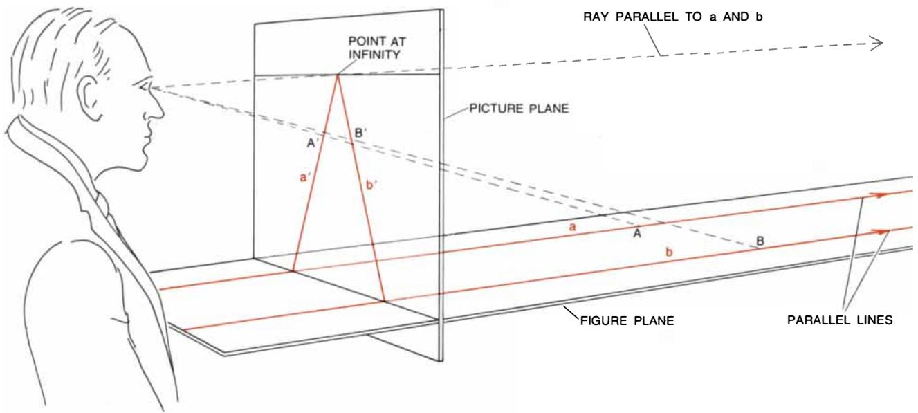
IN PERSPECTIVE DRAWING parallel lines converge at a fictitious "vanishing point" located on the viewer's horizon. The dia-
