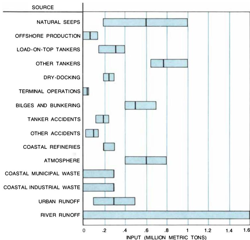
INPUT OF PETROLEUM to the oceans is charted on an annual basis. For each source the black line represents the best estimate and the colored area indicates the probable range.
