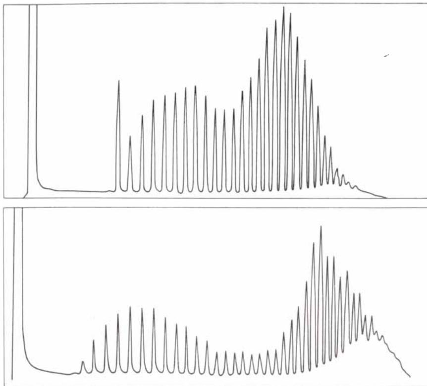
GAS CHROMATOGRAMS of crude-oil sludge (*top*) and pelagic tar (*bottom*) are compared. A chromatograph separates the molecular components of a sample. Here each peak represents a different paraffin molecule of hydrocarbon. The profiles are similar, indicating that the tar originated in crude-oil sludge, which is a waste discharged by oil tankers.
