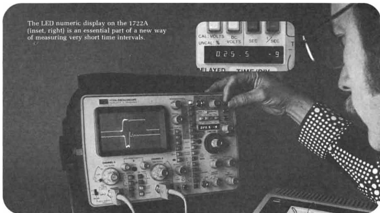
The LED numeric display on the 1722A (inset, right) is an essential part of a new way of measuring very short time intervals.
