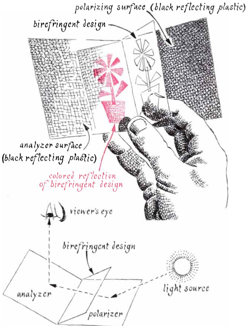
The simple polariscope devised by D. G. Prinz
