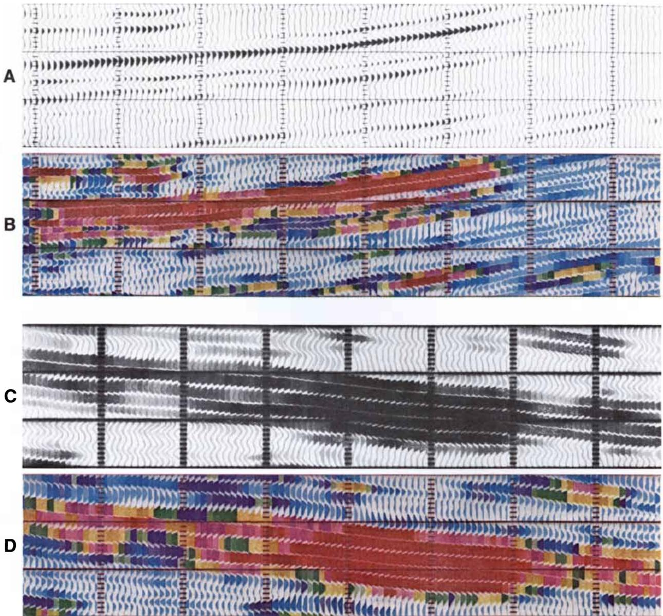
These are fragments of a geophysical “playback” recording from an oil company’s exploration department. A pattern of sensors responded to a shock. The signals were taped. A computer “massaged” the tapes. But need remains for human judgment. The program is not quite capable of typing out a letter to the Finance Committee: “Invest \$[ ] at Latitude [ ], Longitude [ ]. You won’t be sorry.”
