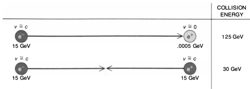
COLLISION ENERGY in electron-positron annihilations depends on the initial energy and momentum of both particles. When one particle is stationary and the other has a velocity near  $c$  (the speed of light in vacuum), the collision energy is only a small fraction of the energy expended in accelerating the moving particle. When two particles collide with equal and opposite velocity, all their energy is made available for the creation of new particles.
