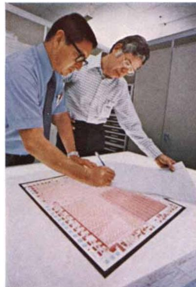
At the Microelectronic Device Division, Bob Larsen (right) and Gerry Lozano verify a set of color masks which represent photoplates used to manufacture microelectronic devices.
