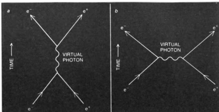
**TWO INTERPRETATIONS** are possible when the product of an encounter between an electron and a positron is another electron-positron pair. The initial pair may have annihilated (a), producing a virtual photon that materialized into an electron and a positron. Or the particles may have passed nearby and been scattered by the exchange of a photon (b).
