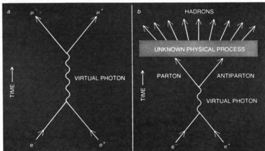
**MUONS AND HADRONS** can be produced in electron-positron encounters only by the annihilation of the particles, not by scattering. The creation of muons (a) requires that the quantum number mu-ness be changed for each of the particles, although the total mu-ness of the pair remains zero. Hadrons are thought to be formed (b) through the creation of a parton and an antiparton (or a quark and an antiquark). The partons interact to form hadrons.
