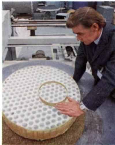
*George Hefferon evaluates mirror optical quality. The honeycomb-like coring greatly reduces mirror weight by eliminating unnecessary glass.*
