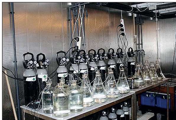
Figure 7.3 Larval cultures at the Sven Lovén ocean acidification facilities (University of Gothenburg). pH is dynamically controlled using pH-computers (Aquamedic) by injection of pure \text{CO}_2 in 5 l closed-circuit aquaria allowing an accuracy of 0.04 pH units (photo credit: S. Dupont).
